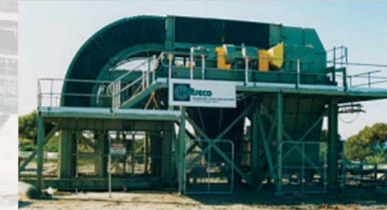
North Head Spoil Removal Project, Vertical Belt Wall Conveyor, Capacity: 650 tph, Location: NSW, Australia
