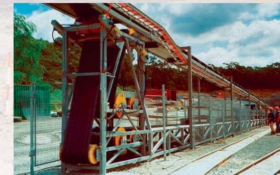
Blue Mountains Sewage Transfer Scheme, Belt Conveyor System, Capacity: 240 tph, Length: 13,000 m Location: NSW, Australia
