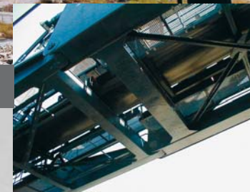
Plomin, Pipe Conveyor, Capacity: 1,250 tph Length: 1,700 m, Location: Plomin, Croatia
