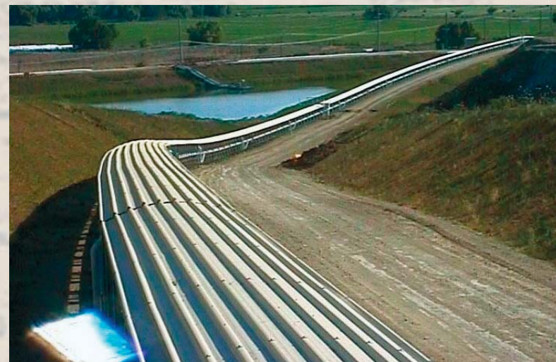
Bengalla, Overland Belt Conveyor System Capacity: 2,000 tph, Length: 4,300 m, Location: NSW, Australia
