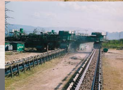
Mae Moh V, Mine Conveyors, Capacity: 2 x 11,000 tph Length: 13,800 m, Location: Lampang, Thailand
