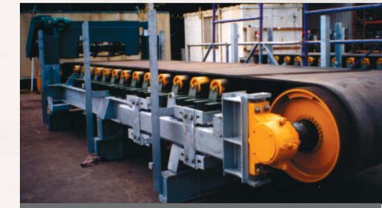
Sun Metals - Zinc Refinery, Belt Feeder Conveyor Capacity: 30 tph, Location: QLD, Australia
