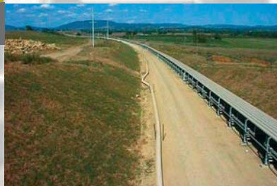
Bengalla, Overland Belt Conveyor System Capacity: 2,000 tph, Length: 4,300 m Location: NSW, Australia
