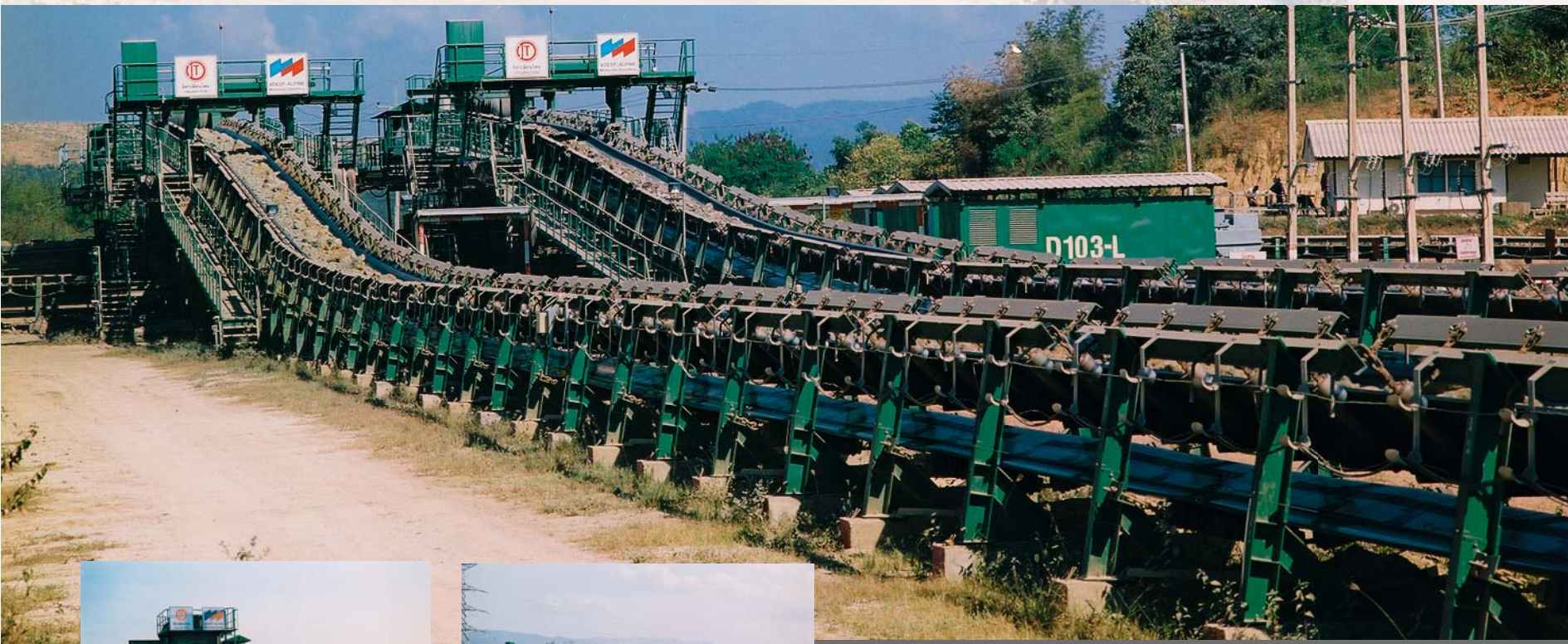
Mae Moh V, Mine Conveyors, Capacity: 2 x 11,000 tph Length: 13,800 m, Location: Lampang, Thailand
