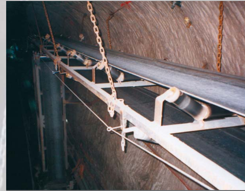
TBM, Spoil Removal Underground Conveyors Capacity: 600 tph, Length: 15,700 m, Location: NSW Australia
