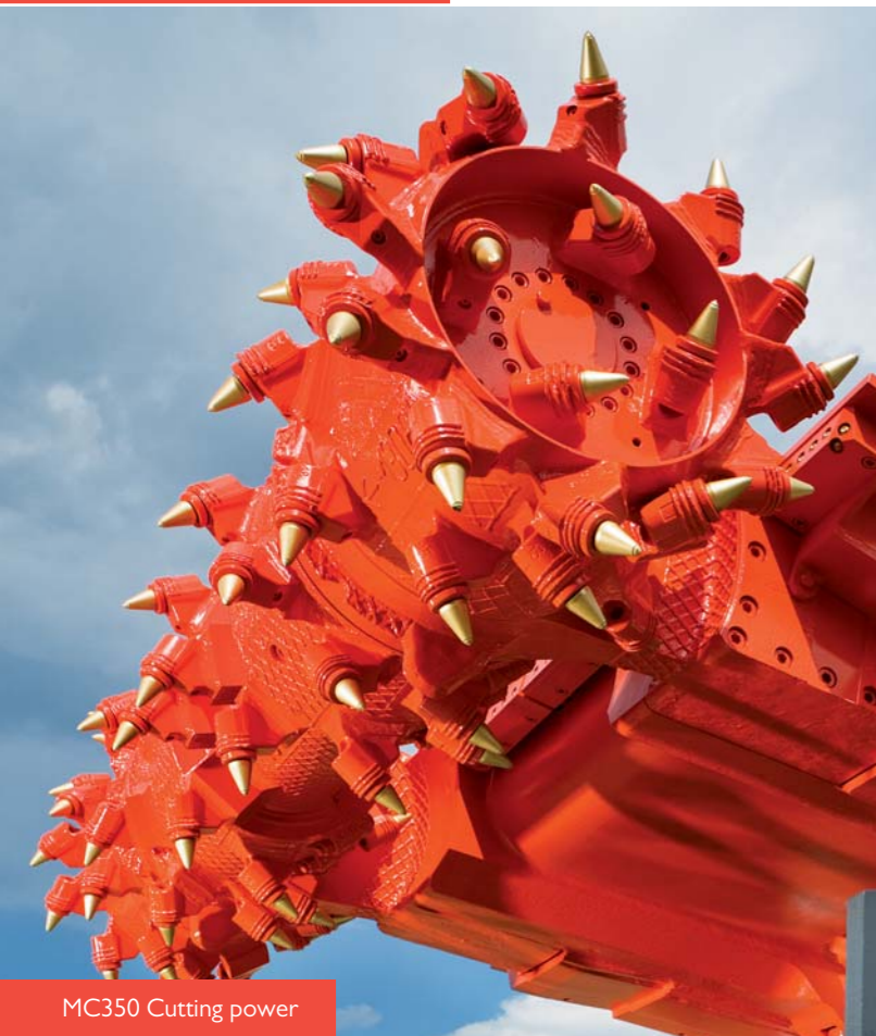
Sandvik Continuous Miner MC350
